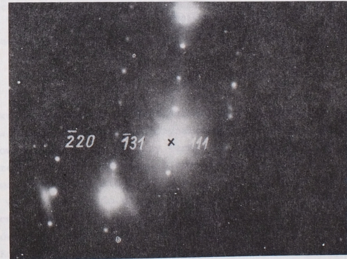
Phot. 7. Electron diffraction of spinel phase microarea with hkl Miller's indices
