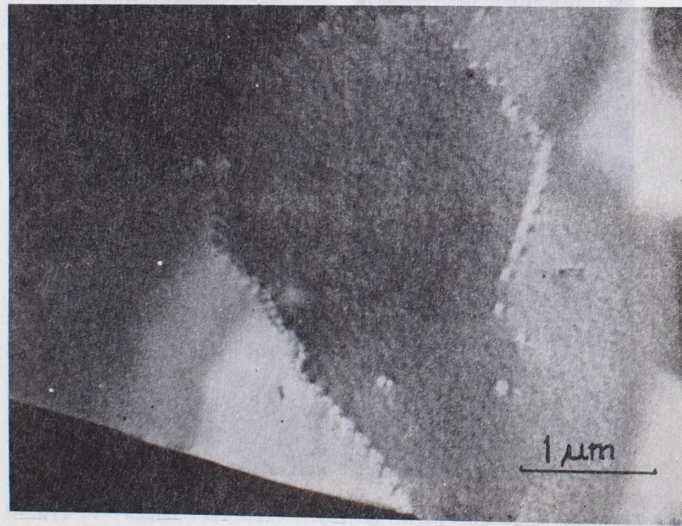
Phot. 5. Electron micrograph performed from spinel phase /C/ microarea with dislocation system /TEM/
